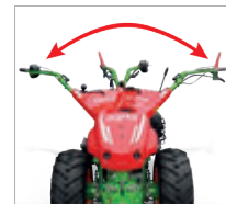
Handlebar can be easily adjusted laterally
