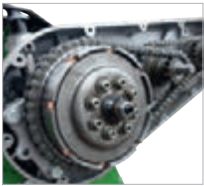
Robust and durable chain drive in oil bath
