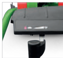
Engine speed adjustable from the steering bar
