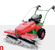
Flexible adjustment of brush pressure
