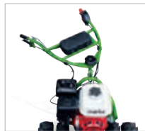
Handle bar laterally adjustable without tools
