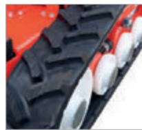
Crawler tracks with non-slip cleat-profile
