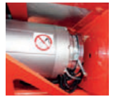
Electromechanical brake for safety on slopes
