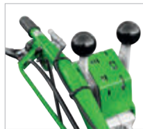
Shift gears and driving direction directly on the handle bar
