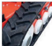
Crawler tracks with non-slip cleat-profile
