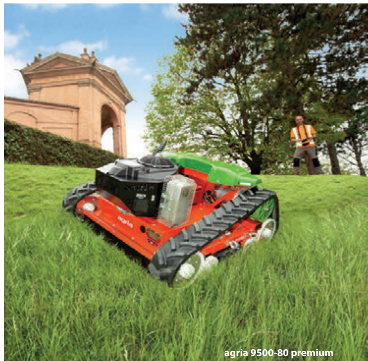
Crawler tracks with non-slip cleat-profile
