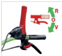
Safe gear change by one-hand operation
