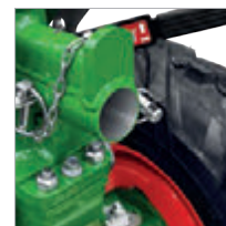
Additional fixture for towed attachments, e.g. ploughs
