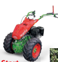
Portal-axle to adjust centre of gravity
