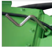
Step- and tool-less height adjustment of handle bar with crank
